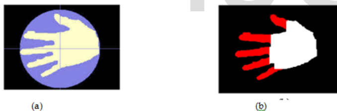
Fig.2. (a) MBC that accommodates the binary hand silhouette inside and (b) finger part and palm part of the binary hand silhouette
